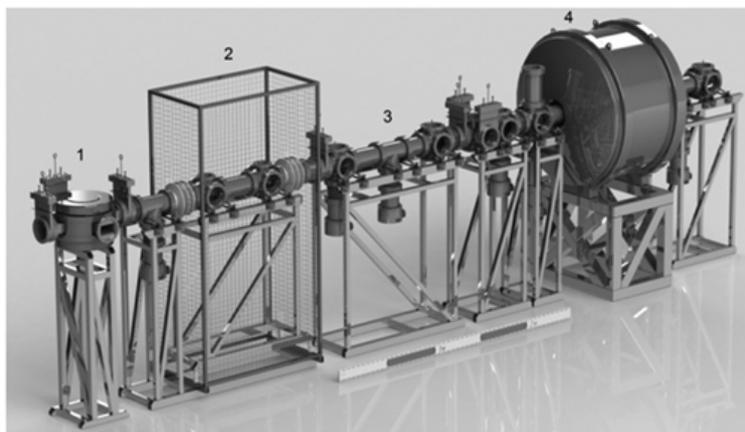
Figure 4. Model of the measuring facility with a Penning ion-trap (4). (1) is a turning magnet, (2) indicates the gas-filled RFQ, (3) is the multi-ToF system.
