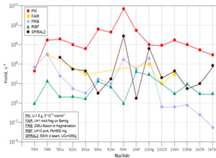
Figure 3. Comparative production yields expected from different on-line installations in the world.
