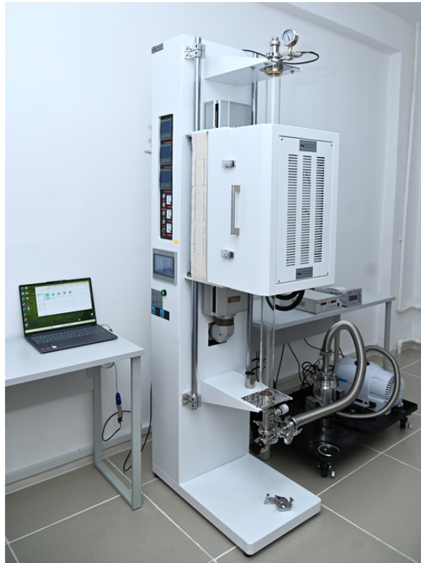
Figure 1. Experimental crystal growth setup implementing the Bridgman method in an argon atmosphere following the establishment of high technical vacuum ( 10^{-6} Torr).
